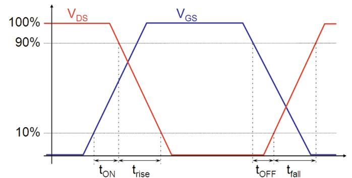
Figure 6. Measuring switching time of a power MOSFET.
