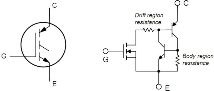
Figure 7. IGBT circuit symbol and equivalent circuit.
