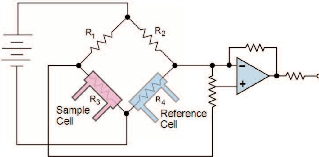
Figure 10. Thermal Conductivity Detector and Wheatstone bridge.
