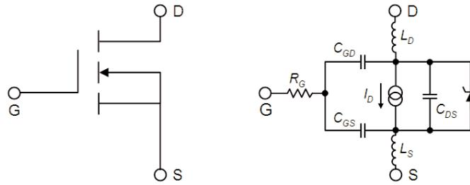
Figure 3. MOSFET schematic and equivalent circuit.
