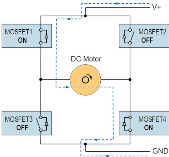
Figure 2. H-bridge configuration of four MOSFETs in a DC-motor drive.
