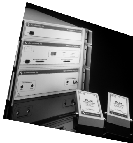
Agilent partners with ATN Microwave to provide load pull systems. Shown here are the electronic load modules (ELM), the electronic mainframe (EM) and a signal conditioning module (SCM) from ATN Microwave that are typically integrated into a load pull system.
