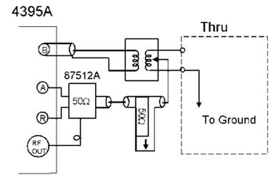
The following figure shows the setup configuration of Isolation calibration for LCL.
