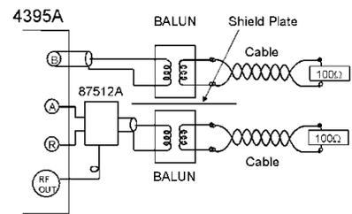
Typically FEXT is measured on installed plant, for example, when the cable is actually installed between a central office and a subscriber. Since it is impossible to connect both ends of the cable to a network analyzer, FEXT is typically not evaluated with a single test instrument.
