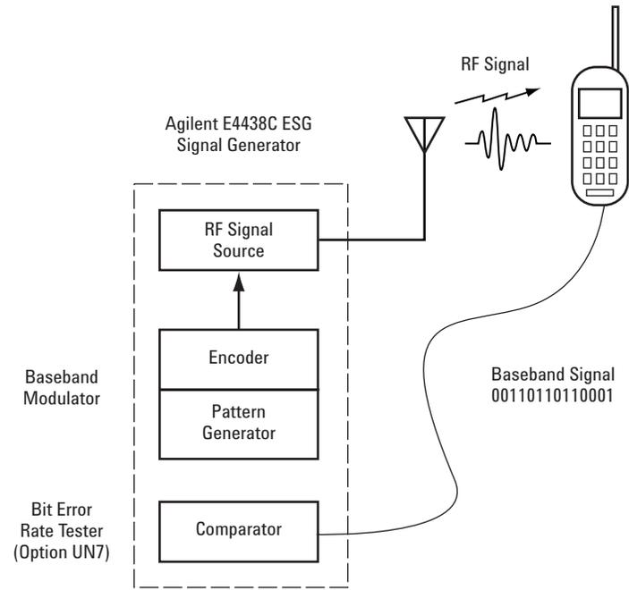
**Figure 7. Loopback BER Test Configuration (this test set-up applies only to GSM/EDGE)**
