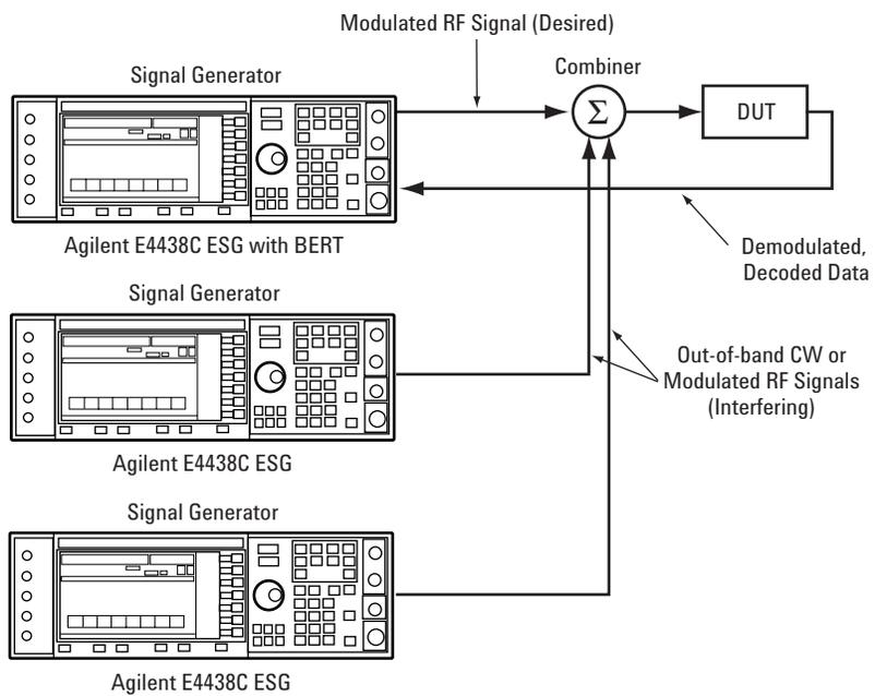
Figure 14. Adjacent and Alternate Channel Selectivity Test Setup
