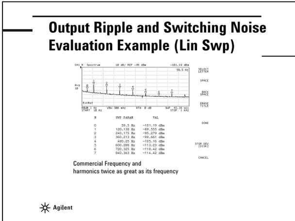
This is an evaluation example of the output ripple and switching noise measurement with linear sweep. You can see the spectrum generated from the power line frequency (60 Hz in this example), with the harmonics twice as large as its frequency (120 Hz, 240 Hz,...).
