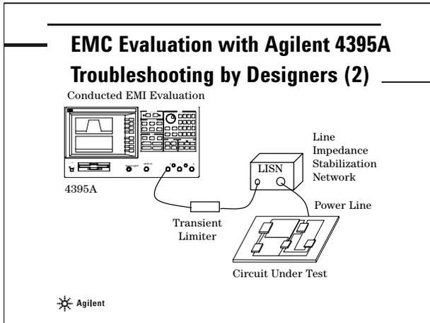
This figure shows an example of the conducted EMI evaluation setup for designers at a laboratory. A line impedance stabilization network (LISN) and transient limiter are connected with the Agilent 4395A. The transient limiter protects the spectrum analyzer input from damage caused by high-level transients from the LISN during EMI testing for conducted emissions.
