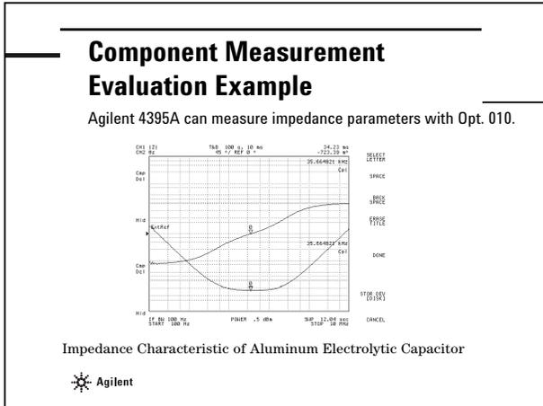
This is an evaluation example of the impedance characteristic of an aluminum electrolytic capacitor. This example displays with the  $|Z|$  and  $\theta$  formats.
