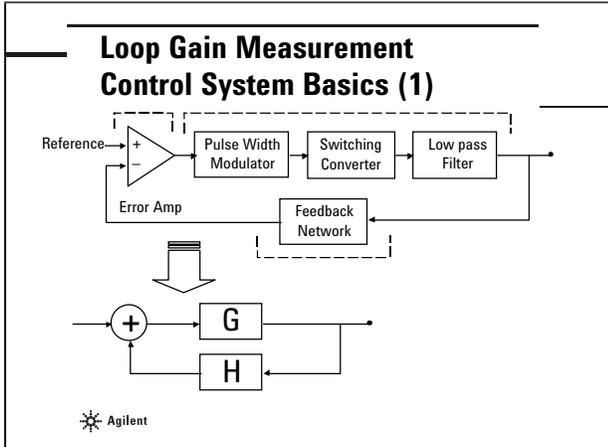
A block diagram of the switching power supply described earlier is shown again in this figure. The position of each box has been slightly changed. This figure shows that the circuit of the switching power supply can be considered as a simple feedback control system.
