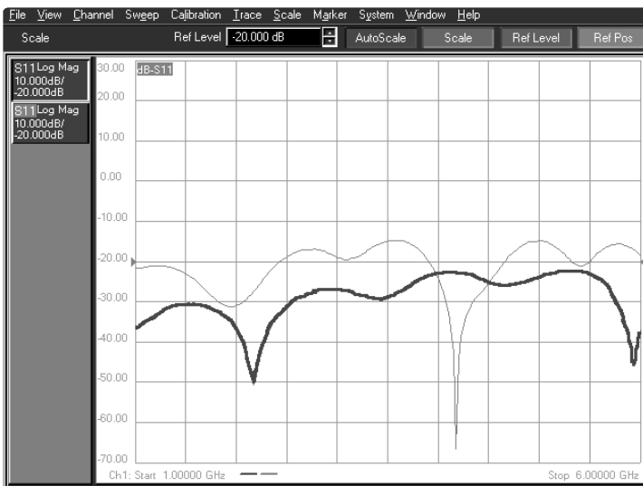
Figure 19. Forward directivity error term (1) using standard coaxial calibration (lower trace) and (2) modified to include the effects of a coax-to-microstrip test fixture (upper trace)
