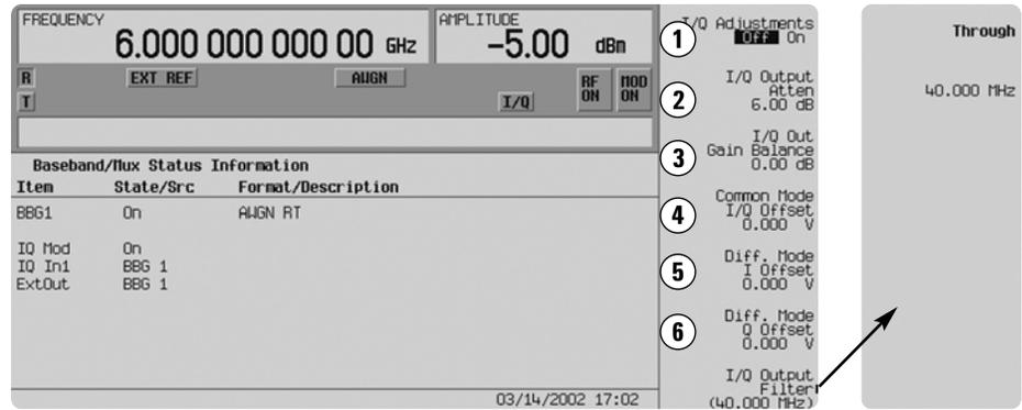
Figure 5. I/Q menu on the E4438C ESG
