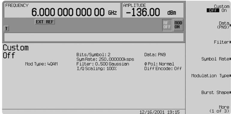
Figure 4. ESG Menu set-up to create a 4 QAM Signal
