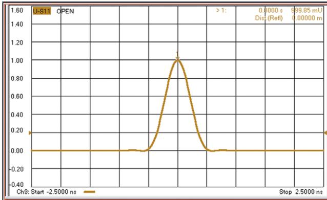
**Figure 37. Impulse response of an open standard.**
