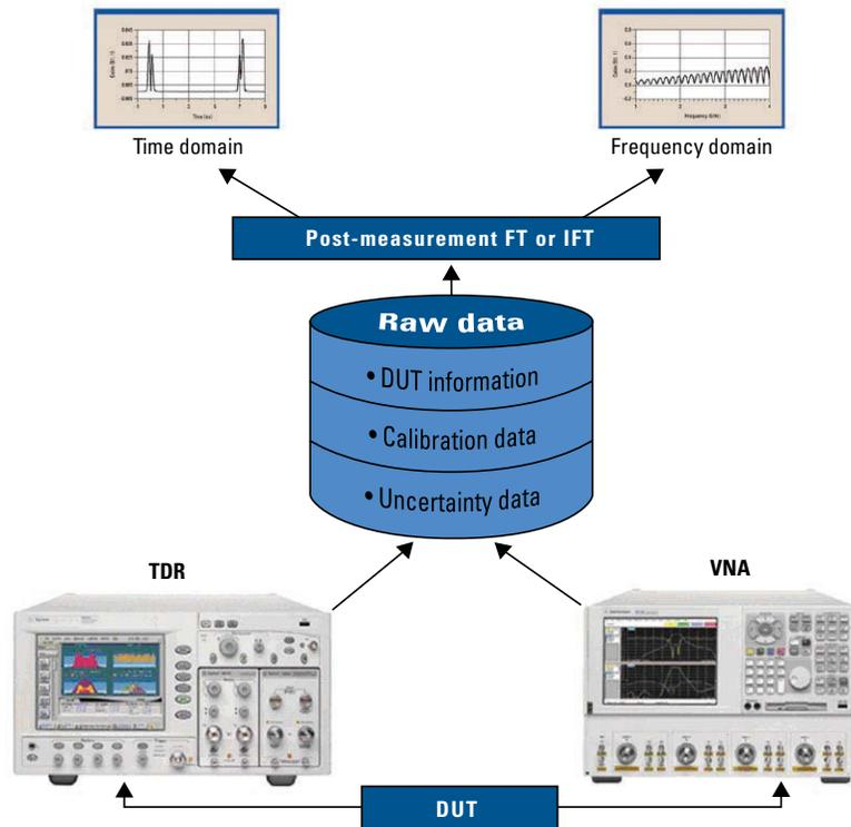
Figure 1. Relationship between time domain, frequency domain, TDR, and VNA.
