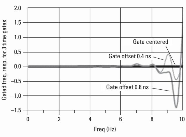
Figure 12c. Frequency response after gating.
