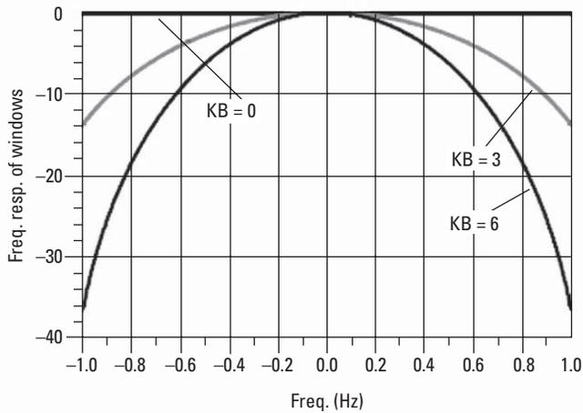
Figure 5a. Applying windowing functions with different  $\beta$  values. Higher values of  $\beta$  reduce the height of the sidelobes. (KB stands for Kaiser-Bessel and is a commonly used window function.)
