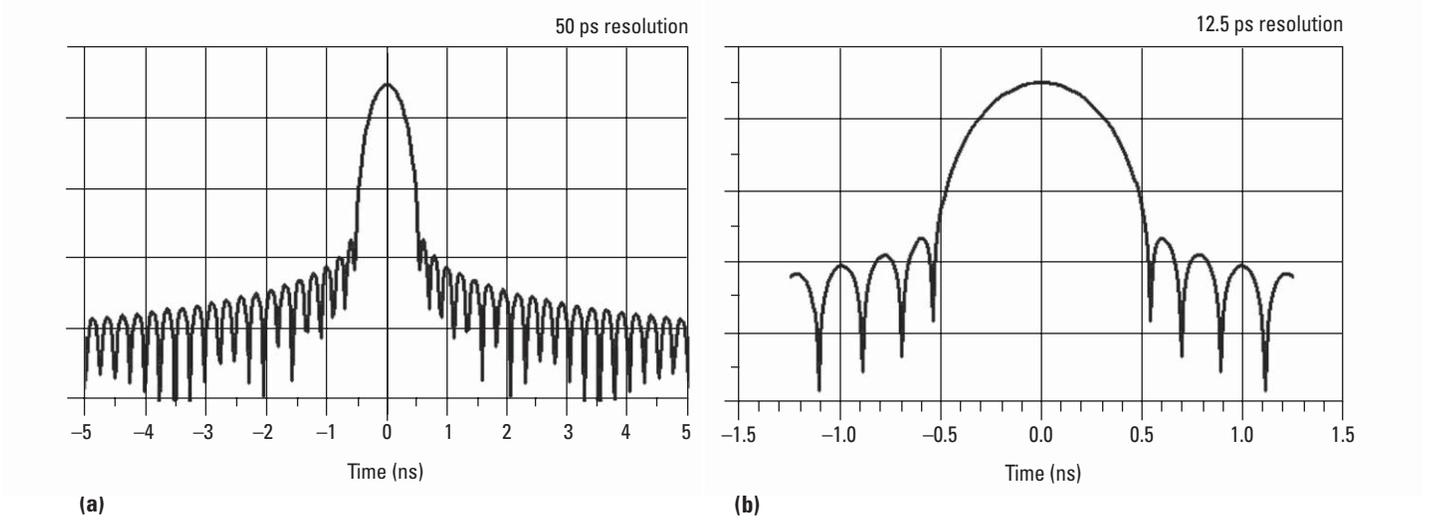
**Figure 27. Range resolution: (a) a span of 10 ns results in a range solution of 50 ps, (b) reduce span to 2.5 ns and reduce resolution to 12.5 ps.**
