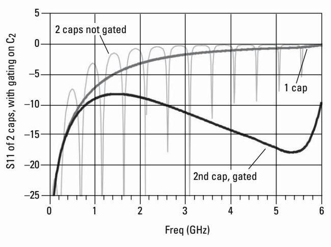
Figure 18. Gating out the second discontinuity (circuit shown in Figure 16).
