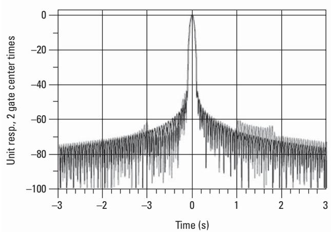
Figure 12b. A unit frequency response in the time domain with gates applied at various gate times.
