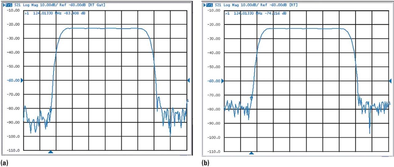
**Figure 34. Effect of gating on and off: (a) with gating on, the effect of RF leakage and triple travel signal have been removed, and the result is an improvement in out-of-band rejection, (b) no gating applied (same as Figure 29).**
