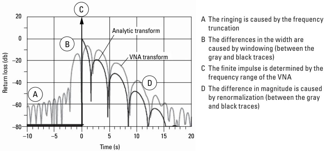
Figure 2. Comparing IFT calculated (analytic transform) and VNA time domain transform of the same function.
