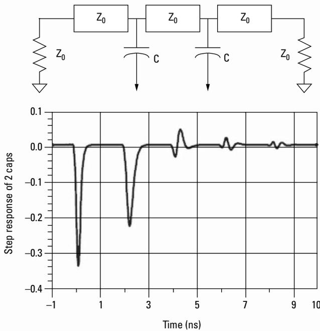
**Figure 20. For two discrete identical discontinuities, response of the second discontinuity is somewhat masked by the first because not all energy reflected from the first discontinuity is available to be incident on the second.**
