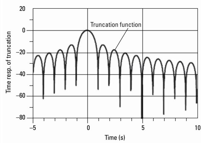
Figure 4b. Truncation causes ringing in time domain.
