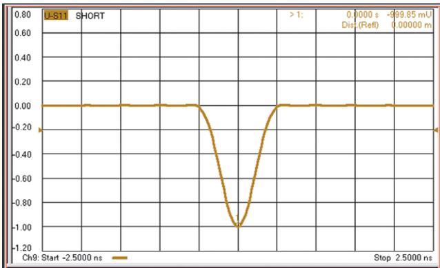
**Figure 38. Impulse response of a short standard.**
