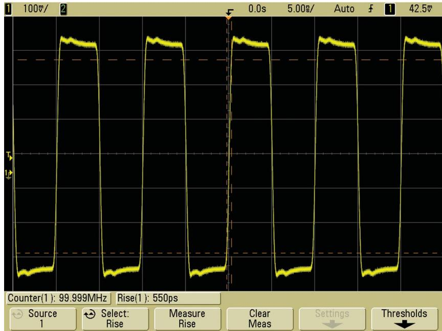
Figure 5: 100-MHz clock captured on the Agilent MS07104A 1-GHz bandwidth scope
