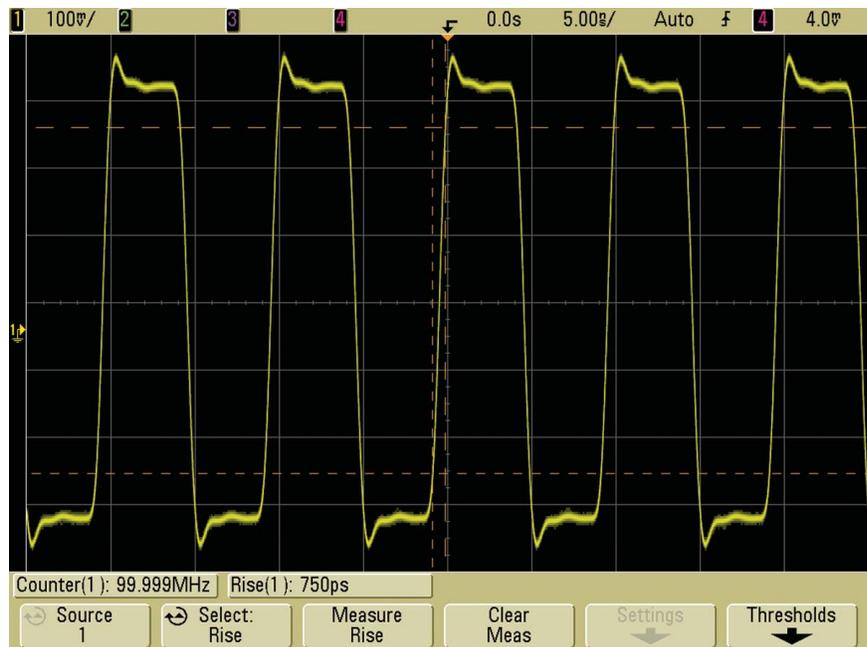
Figure 4: 100-MHz clock captured on the Agilent MSO7054A 500-MHz bandwidth scope
