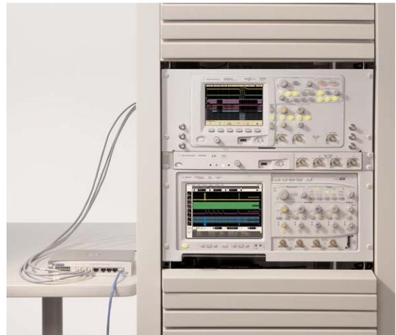
intentionally chose to leave a few slots empty for future enhancement or extension. With LXI, future test system additions will be easier and the system will consume only the space you need.
