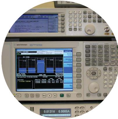
Every millisecond counts when testing the semiconductor devices used in cellular phones. For one multinational manufacturer, an LXI-based test system shaved 2800 ms off the time required to test W-CDMA power amplifier ICs. That time savings has the potential to provide a 233.3 percent increase in daily throughput compared to a GPIB-based system.
