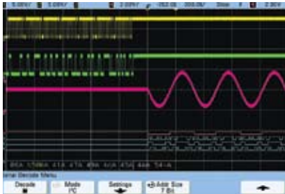
Use MSO digital channels to debug control signals and data buses.
