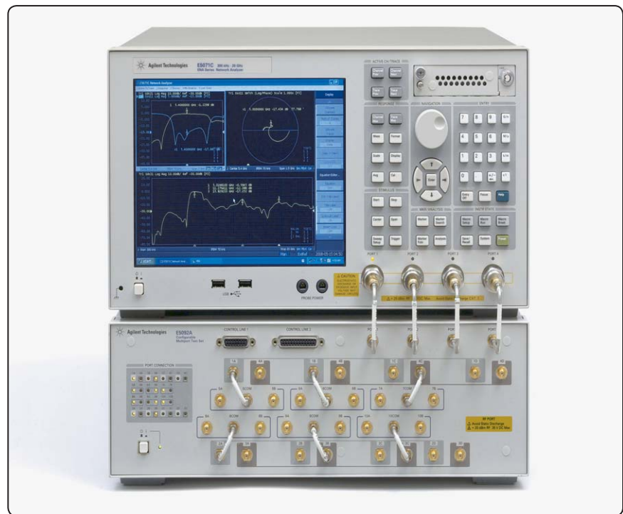
Figure 4. Cable connection for the 22-port configuration 1
