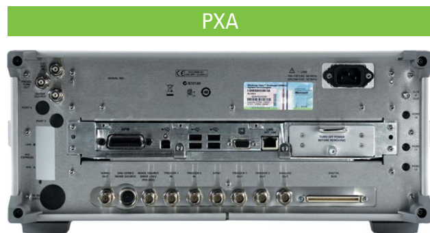
Figure 24. PXA rear panel
