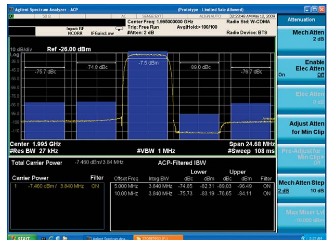
Figure 10. A PXA W-CDMA ACLR measurement showing -89 dBc dynamic range
