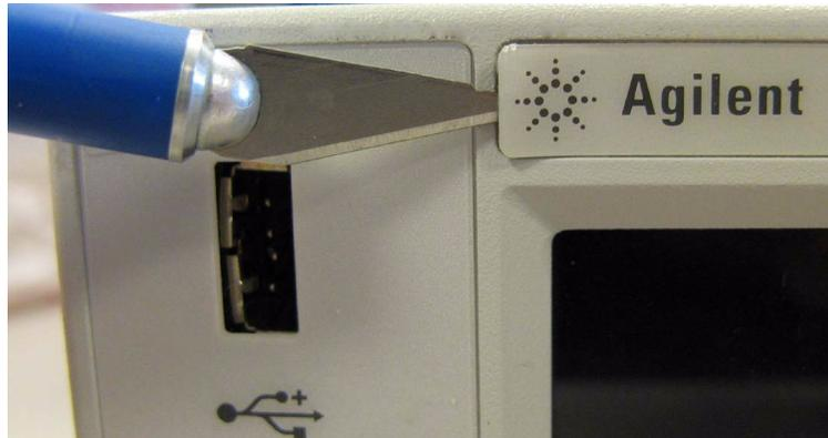
2. Pull the lifted end to remove the nameplate.
