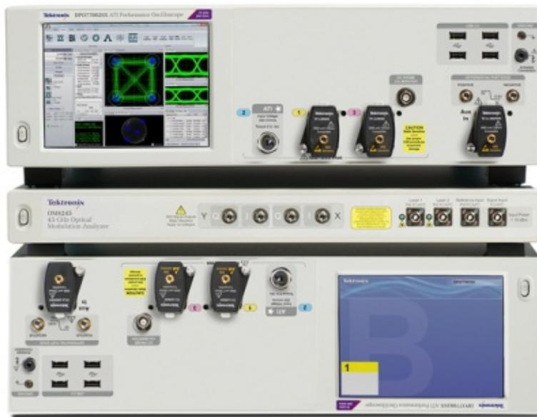
Figure 8: The DPO70000SX is designed so that one unit can be inverted so that ATI ports can be located near the DUT for shorter cables to preserve signal fidelity.
