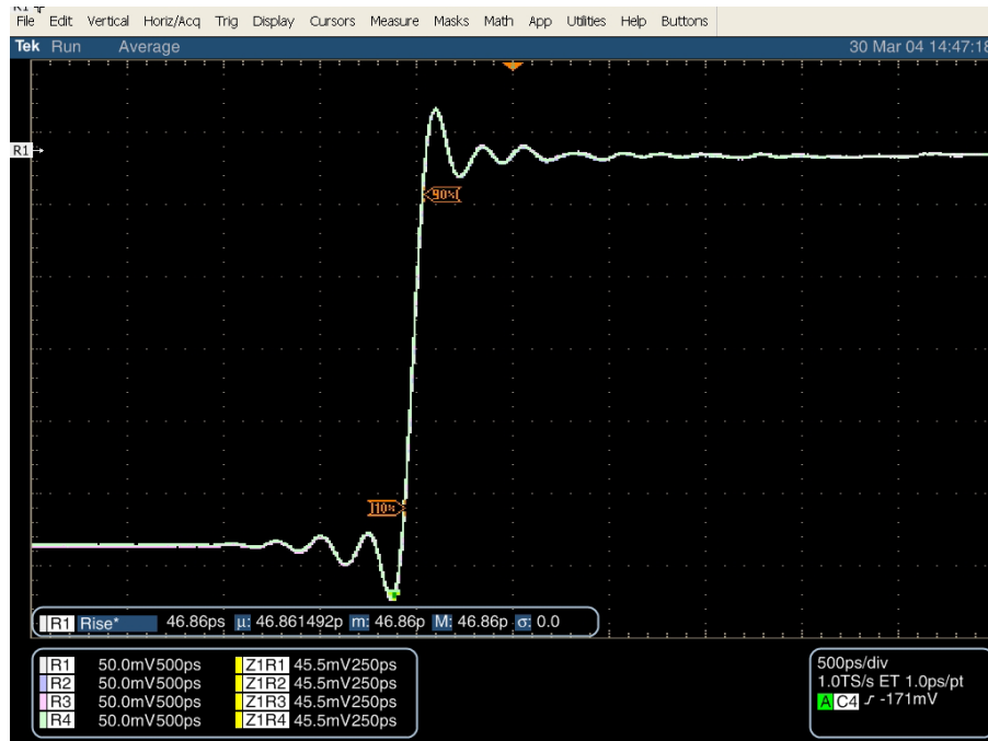
Figure 7. All four channels overlaid with B_{W+} turned on and deskew adjustment made to time align. Risetime readout using 10% to 90% is 46.86 ps using a 15.5 ps step generator. An average of 500 was used (8 GHz bandwidth).
