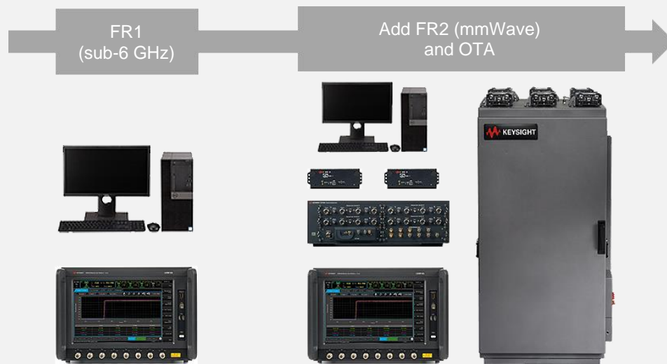
Figure 19. 5G FR2 mmWave test setup
