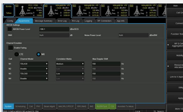
Figure 9. Channel emulation support for baseband fading
