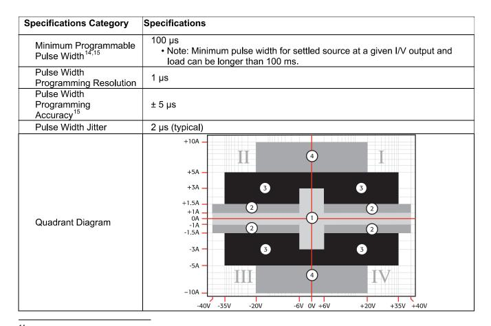
Typical performance for minimum settled pulse widths: Typical tests were performed using remote operation, 4W sense, and best fixed measurement range. For more information on pulse scripts, see the Series 2600A Reference Manual.
