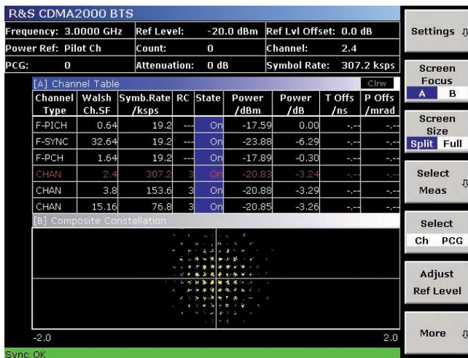
The upper part of the screen shows an overview of the detected channels and a number of parameters such as power and timing offset. The lower part shows the composite constellation diagram of the signal.
