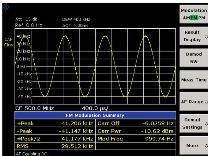
Frequency deviation measurement: display of modulation signal together with peak and RMS deviation, carrier frequency offset and carrier power.
