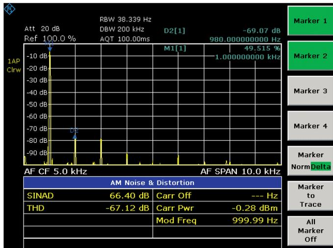
THD measurement on an amplitude-modulated signal: The first harmonic of the modulation signal is well suppressed by 69 dB. This corresponds to a THD (D2) of less than 0.1%.
