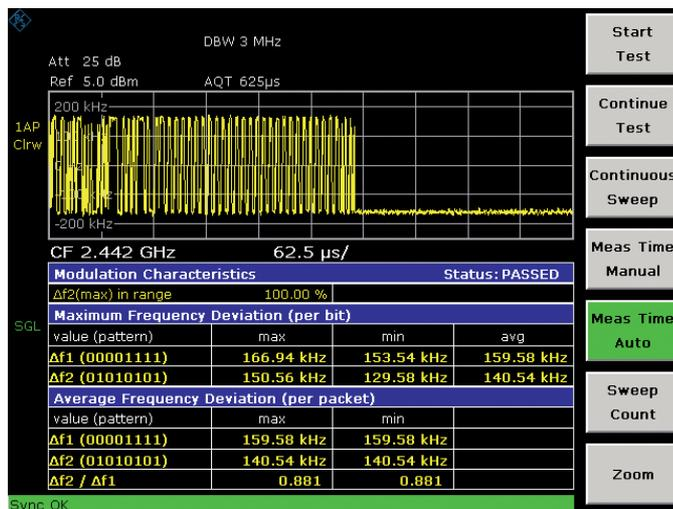
**Modulation characteristics:** This measurement determines the maximum frequency deviation of all 8-bit test sequences of the payload. In addition, the average value of the maximum frequency deviations per packet is calculated and displayed.
