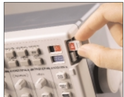
Application Module being installed.
