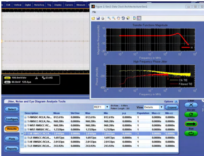
Example of RefClk measurements, together with generated plots
