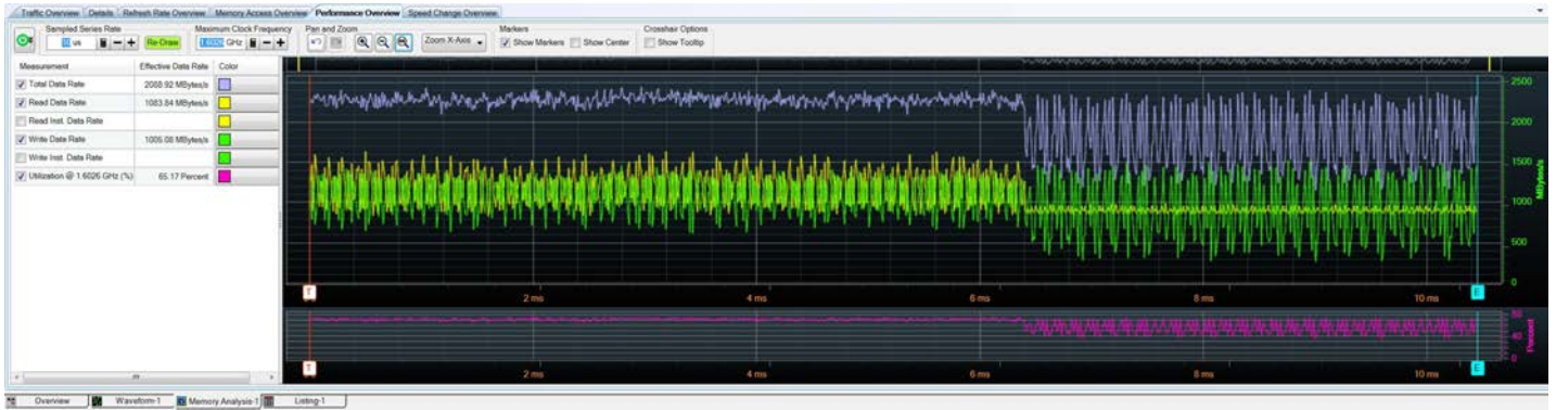
Figure 18. Performance analysis overview. B4661A Option-4FP/-4NP/-4TP provides data rate performance and percent utilization analysis and graphs.
