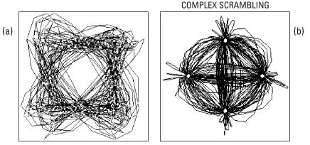
Figure 7. Constellation of (a) an OQPSK signal versus (b) a QPSK signal with basic complex scrambling (Agilent Technologies E4406A VSA series transmitter tester screen displays)
