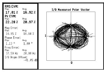
Figure 23. EVM (uncoded) and constellation for a W-CDMA signal with an I/Q gain impairment (E4406A VSA series transmitter tester display)
