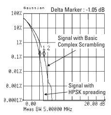
Figure 18. CCDF comparison between signals with and without HPSK (E4406A VSA series transmitter tester display)
