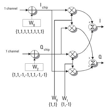
Figure 9. HPSK: Complex scrambling with Walsh rotator and evennumbered Walsh codes
