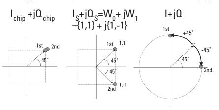
Figure 8. Complex rotator rotates first and second chip points by +45° and -45°, respectively
