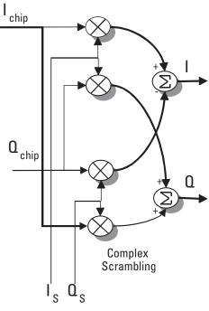
Figure 3. Complex scrambling block diagram
