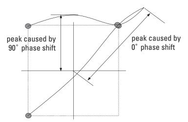
Figure 11. 0° phase shift transitions cause higher signal overshoot
