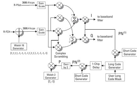
Figure 17. Proposed reverse link structure for cdma2000 SR3 systems
