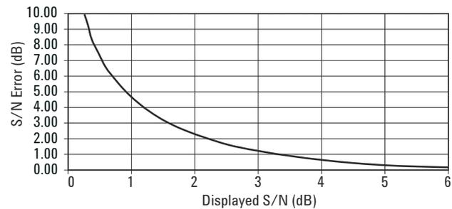
To use the graph shown in Figure 2-14, locate the displayed signal-to-noise ratio on the x-axis, then read off the error on the y-axis. Subtract this error value from the displayed signal amplitude to compute the true CW signal amplitude. For example, suppose the displayed S/N is 3 dB for a displayed signal measuring -100 dBm. The corresponding error is 1.1 dB, which means that the true signal amplitude is -100 dBm minus the 1.1 dB error term, or
