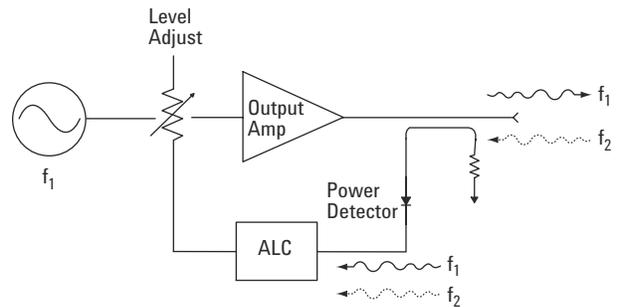
The solution to improving source generated IMD is to prevent the energy of the second source signal from entering the output port of the signal source. The required isolation between the two sources is dependent on the susceptibility of the signal source to signals entering the output port as well as the acceptable AM sideband level needed for the TOI measurement.
