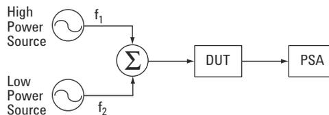
monitored by the spectrum analyzer while the other tone at a much higher power level drives the DUT into gain compression. When in gain compression, the amplitude of the lower power tone decreases by the gain compression value (that is, for a 1 dB gain compression measurement, the amplitude of the lower power tone is 1 dB lower than when the higher power tone is turned off). When the desired gain compression is reached, the amplitude of the higher power tone is measured by the spectrum analyzer.
