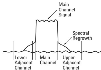
power across the entire main channel and each of the adjacent channels. In either case the user must set the proper mixer level of the spectrum analyzer to minimize the internally generated spectral regrowth. However, minimizing internally generated spectral regrowth comes at the price of increasing broadband noise, therefore a balance
