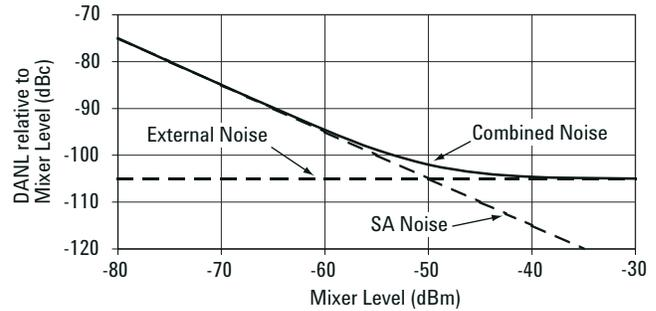
external noise curves, the combined noise is 3 dB higher than the two individual contributors alone. The external noise as displayed on the spectrum analyzer follows the same dependency on RBW setting as the SA noise, such that for every decade increase in RBW value, both the SA Noise and the external noise curves shift up by 10 dB on the dynamic range chart.
