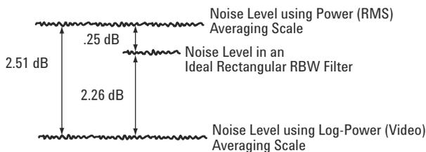
Figure 2-4 shows the relationship between noise, displayed noise using the Log-Power (Video) scale, and displayed noise using the Power (RMS) scale.
