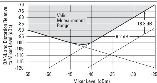
Thus in order to drive down measurement error, the loss in dynamic range is 6.1 dB and the optimum mixer level is shifted down in power by 6.1 dB.
