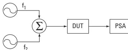
This procedure focuses on the measurement of third order IMD for two CW tones present at the input of a DUT. In a similar vein to the harmonic distortion measurement procedure, the suggested configuration ensures that IMD products generated by the analyzer are at least 18 dB below the IMD products of the DUT. Again, this guarantees that the distortion measurement error due to internal distortion added to DUT distortion is less than 1 dB.
