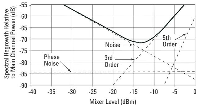
The frequency offset value used to approximate the phase noise results from the following computation: the half-bandwidth of the measurement channel is  $(1.23 \text{ MHz} / 2)$ , or 615 kHz. At a measurement frequency 885 kHz away from the center of the main channel, the frequency difference between the measurement frequency and the edge of the main channel is 885 kHz minus 615 kHz, or 270 kHz.
