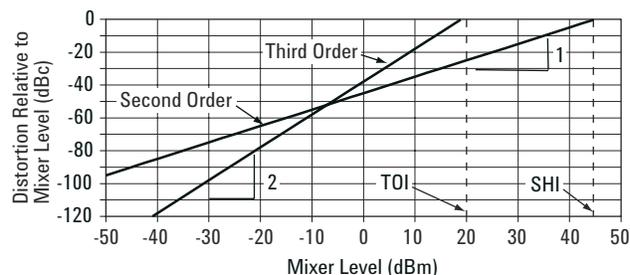
For second order distortion the slope of the S/D versus mixer level curve is +1, signifying that for every 1 dB increase in power at the mixer, the S/D decreases 1 dB. For third order the slope of this curve is +2; for every 1 dB increase in the two fundamental tone power levels, the S/D decreases by 2 dB. For the second harmonic curve the 0 dBc
