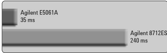
Agilent E5061A verses Agilent 8712ES sweep speed comparison with typical data (201 points, full 2-port cal., 90 dB dynamic range).
