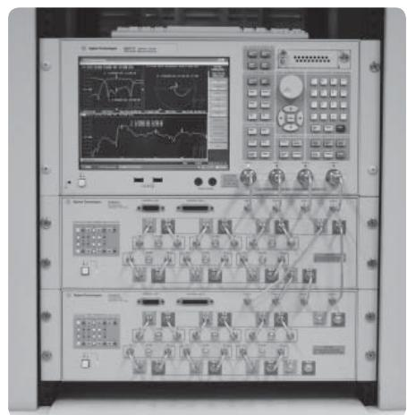
Figure 29. Two E5092A configurable test sets cascaded
