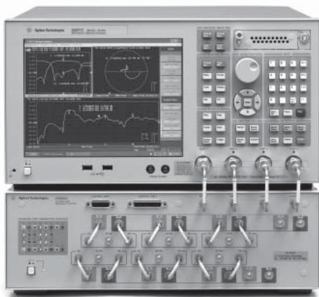
Figure 27. Connection of external cables for a 10-port full crossbar configuration
