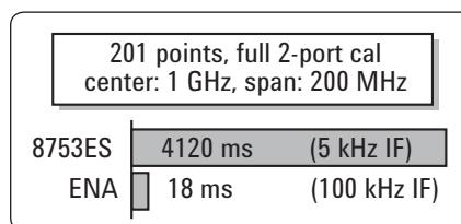
Figure 3. Speed comparison at 0.01 dB p-p trace noise
