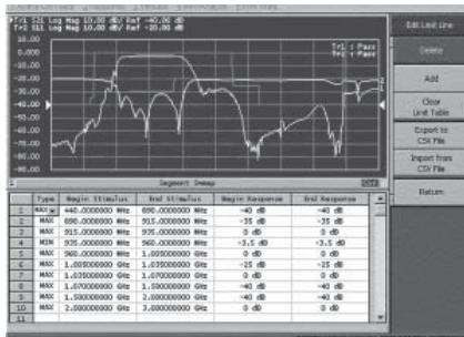
Figure 6. Setting limit line using spreadsheet
