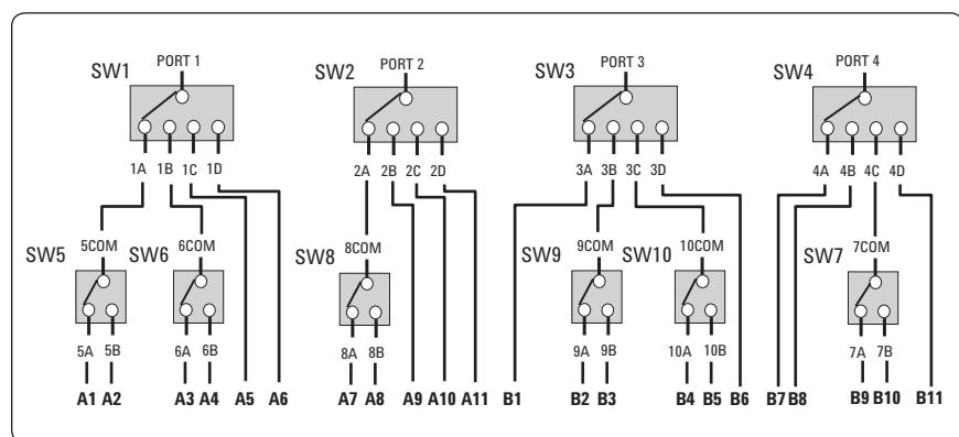
Figure 24. Block diagram of 22-port configuration
