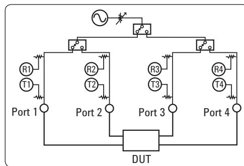
Figure 23. 4-port ENA hardware architecture
