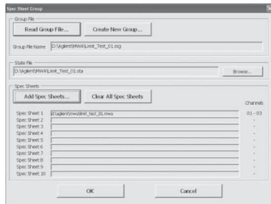
**Figure 33.** The .mwa setup file sets all the measurement parameters on the ENA automatically
