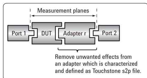
**Figure 20. De-embedding for mixed-connector device measurements**
