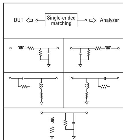
**Figure 22. Pre-defined models of matching circuit embedding**
