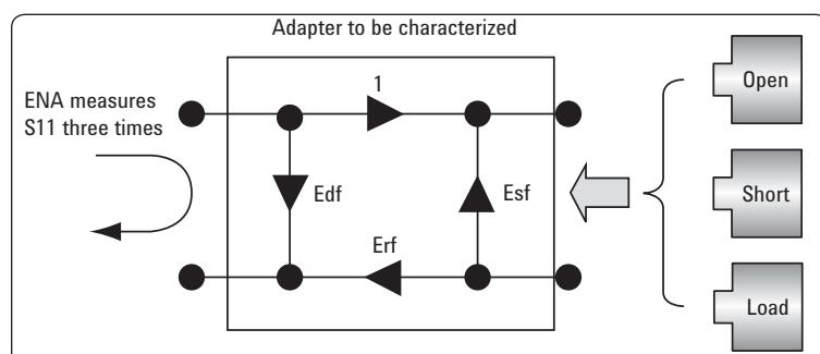
Figure 14. Adapter characterization (single directional method)
