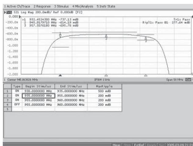
Figure 11. Ripple limit test
