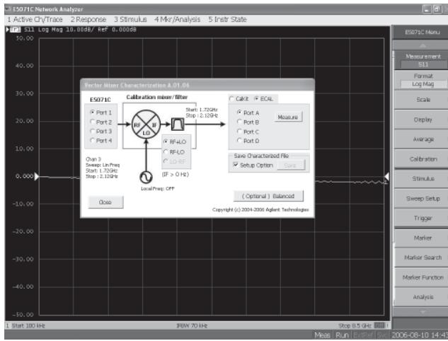
Figure 36. Vector-mixer calibration using VBA
