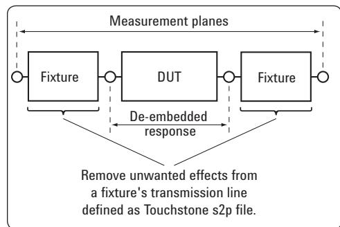
**Figure 19. De-embedding for removing fixture effects**
