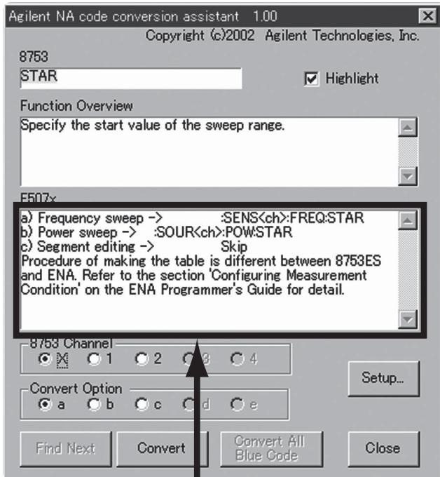
Figure 39. Quick Help shows equivalent GPIB commands and code conversion tips
