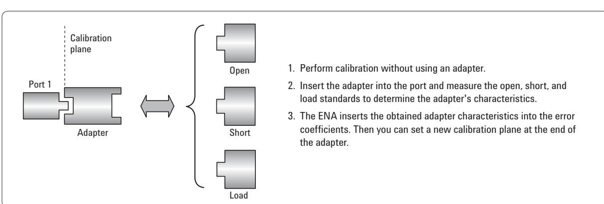
Figure 16. Enhanced adapter removal and insertion
