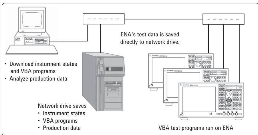
Figure 9. ENA factory automation example
