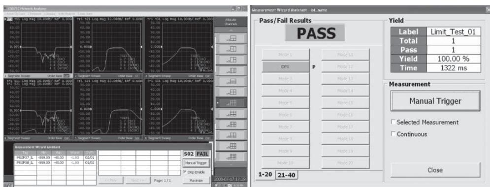
**Figure 35.** Automatic test procedures provide go/no go limit testing
