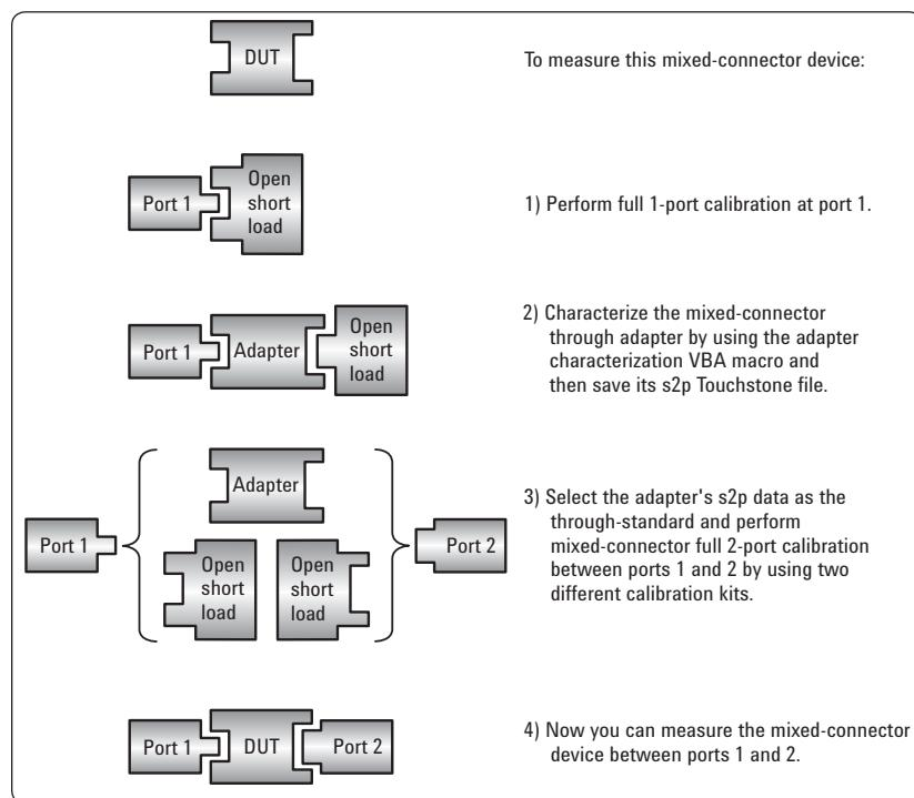
Figure 13. Mixed-connector calibration using adapter characterization (in the case of 2-port measurement)
