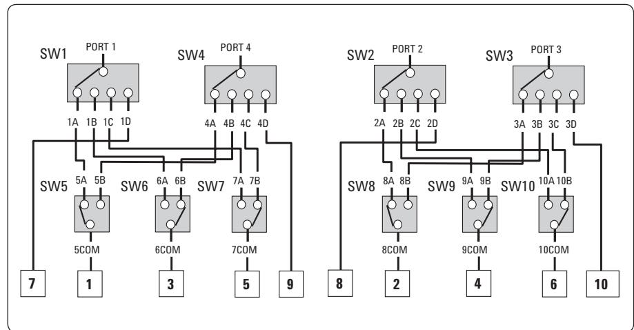
Figure 26. Block diagram of 10-port full crossbar configuration
