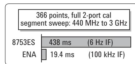
Figure 4. Speed comparison in high-volume manufacturing
