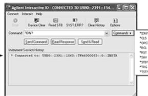
This step shows how to send SCPI commands to 34405A DMM and read responses using the Interactive IO.
