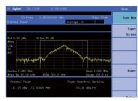
Figure 1 Channel power measurement
