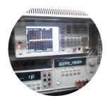
Figure 4 Testing system – N9320B RF spectrum analyzer, E3632A power supply and 34401A digital multimeter
