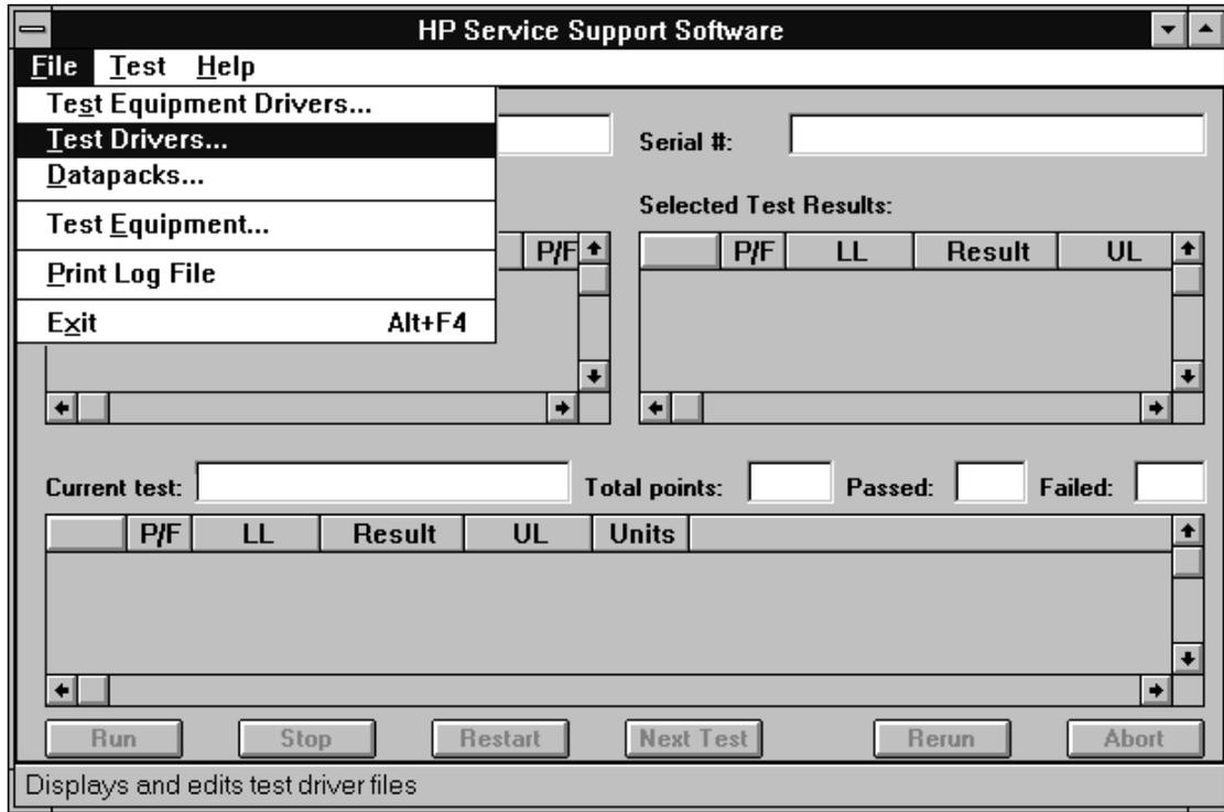
2. Refer to [Figure 3-11](#). To add a test driver to the existing list of test drivers, click Add.
