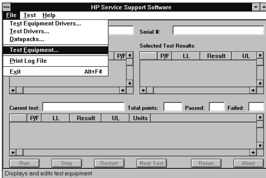
2. Refer to [Figure 3-3](#). In the Test Equipment dialog box, select the Device Type for the new equipment you are adding.
