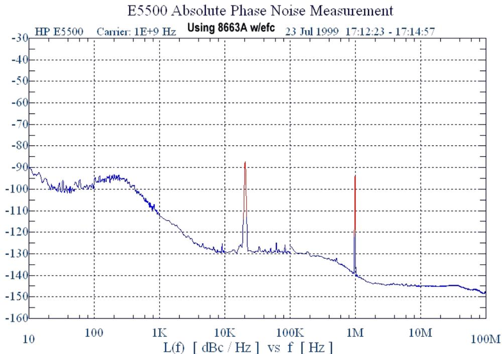
To get an accurate idea of the actual phase noise of the DUT, it may be necessary to combine the two plots, always using the lowest result of both (see Figure 4-37). Keep in mind that the actual phase noise results are probably better than what is displayed.
