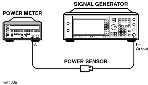
**Figure 4-20 Low-Power, Power Level Accuracy (< 10 MHz) Setup**
