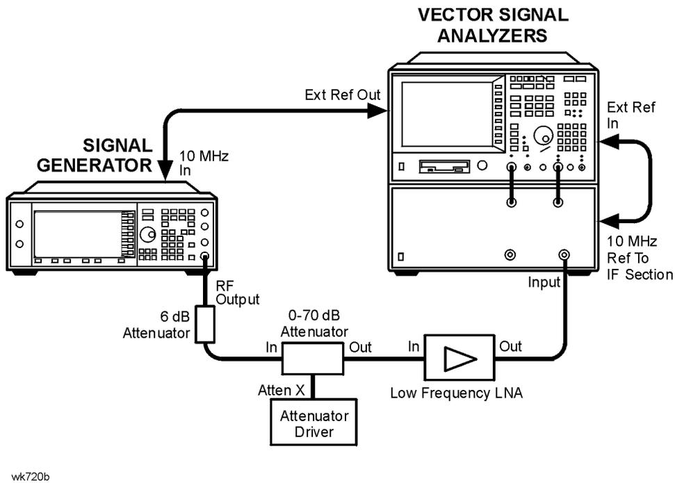
**Figure 4-21 Low-Power, Power Level Accuracy ( $\geq 10$  MHz and  $\leq 2$  GHz) Setup**
