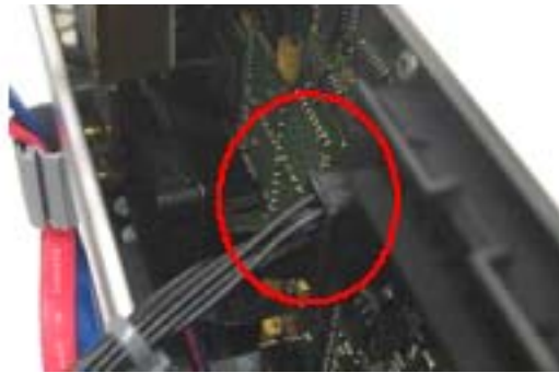
Front panel power cable connector
