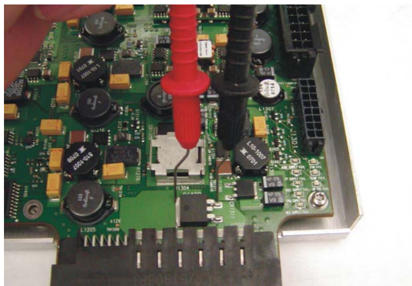
Measuring the backplane assembly resistance between +12 V and ground across Q1409
