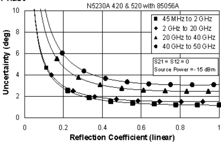
**Table 10. 85056A Calibration Kit****N5230A/C- Option 425 or 525 (Configurable Test Set and Extended Power Range)**
