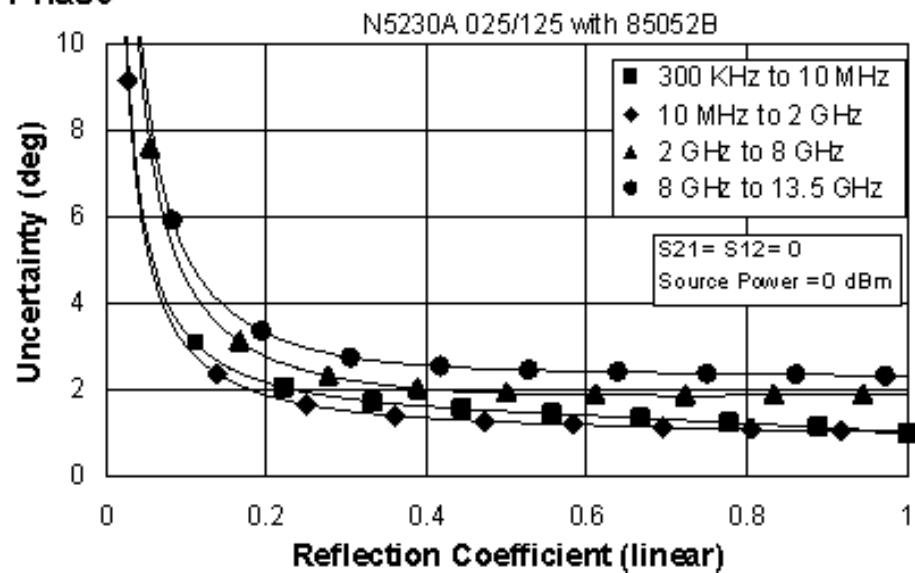
**Table 5. 85052B Calibration Kit****N5230A/C- Option 220 (Standard Test Set and Standard Power Range)**
