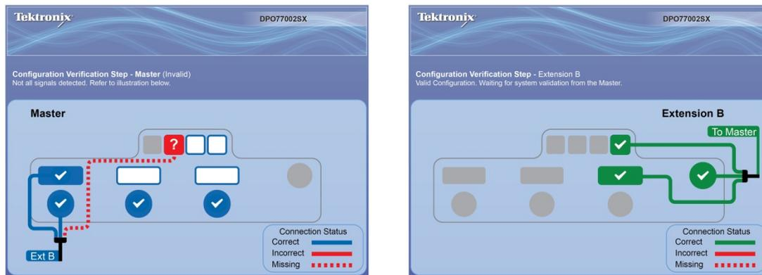
Figure 5: The UltraSync configuration manager coordinates multi-unit startup and verifies connections.
