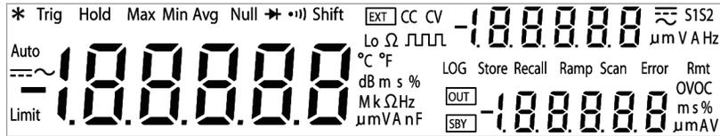
**Figure 1-5** VFD full display with all segments illuminated
