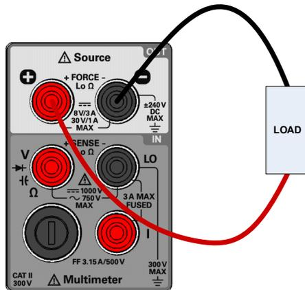
**Figure 3-1** Constant voltage mode terminal connections
