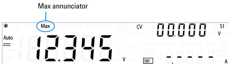
Press **MinMax** again to step through the maximum reading (the Max annunciator is illuminated), minimum reading (the Min annunciator is illuminated), average reading (the Avg annunciator is illuminated), or present reading (the MaxMinAvg annunciator is illuminated).
