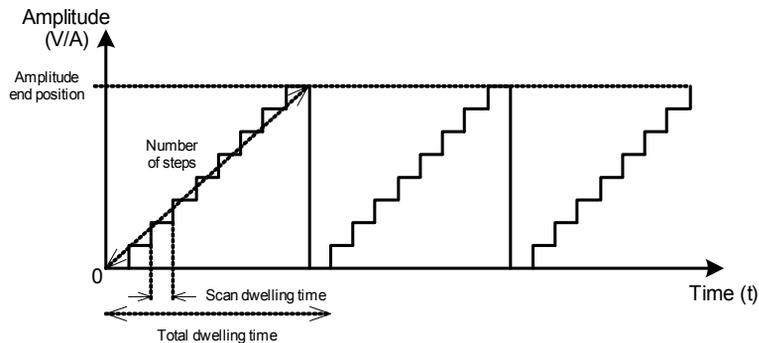
The total dwell time will increase with respect to the number of steps and the scan dwell time per step selected. The scan dwell time is defined as the length of time the scan signal will “dwell” in the present step before incrementing to the next step.
