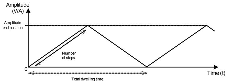
The ramp dwelling time will be set to the fastest of the instrument capability (typically ~300 ms per step). A higher number of steps provides a more linear ramp signal. This however will result in an increase in the total dwelling time. A lower number of steps will result in a shorter total dwelling time and a more stepped ramp signal.
