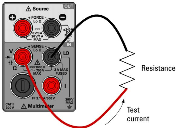
Figure 2-3 Terminal connections for 2-wire resistance measurements
