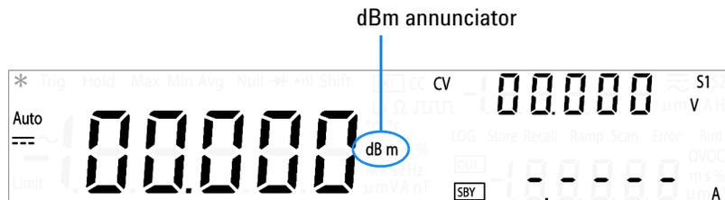
Press **Shift** > **dBm** again or **Shift** > **Exit** to exit the dBm mode.
