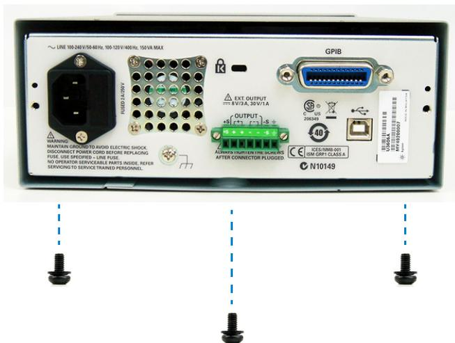
**6 Slide the cover off the instrument.**
