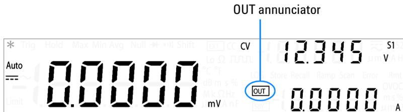
The  $\frac{\text{OUT}}{\text{STBY}}$  key is also used to generate the square-wave output at the selected amplitude, frequency, pulse width, and duty cycle.
